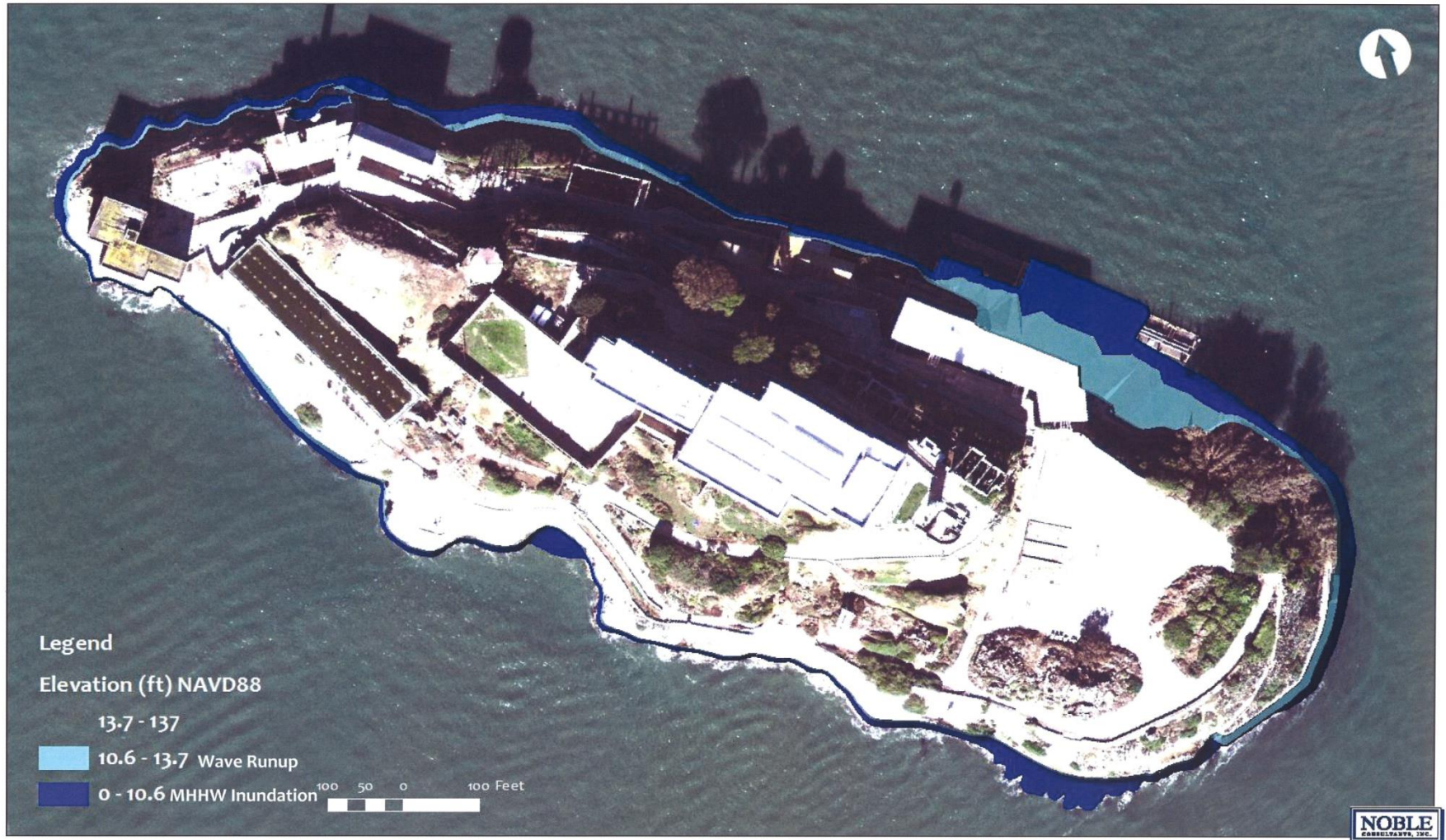
Figure 9. Overview of inundation (10-yr water level=10.6 ft) and potential wave runup zones based on Sea Level Rise estimates in the year 2060 (50 yrs).
