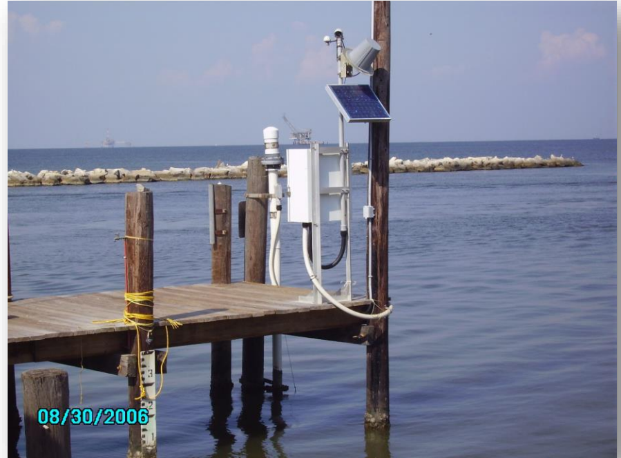
NOAA water level monitoring station with an acoustic sensor on Dauphin Island, Alabama.
